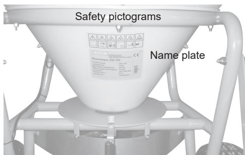
Figure 2.1: Name plate, safety pictograms
